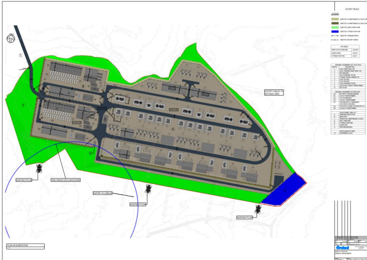
Figure 4.22: Indicative 2D plan view of Onshore HVAC Substation layout with the Energy Balancing Infrastructure (North-West) and Attenuation Feature in blue (South-East).
